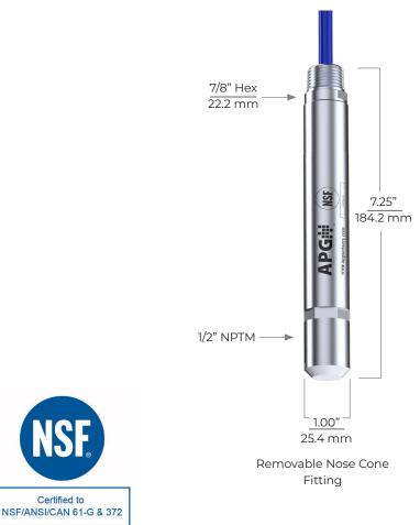
The PT-500E is a rugged submersible pressure transmitter specially designed for potable water applications requiring NSF certifications and can be used in other tank liquid level measurement, water and wastewater applications, and well depth measurement.
