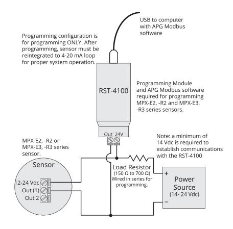
● IMPORTANT: MPX level sensor MUST be installed according to drawing 9003468 (Hazardous Installation and Non-Incendive Wiring Drawing) in section 9 to meet listed approvals. Faulty installation will invalidate all safety approvals and ratings.
