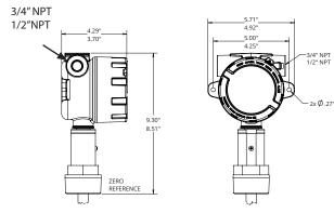
Note: for dual dimensions, large housing dimensions are above small housing dimensions.
