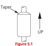
**⑤** IMPORTANT: Floats must be oriented properly on the stem, or sensor readings will be inaccurate and unreliable. Untapered floats will have a sticker or "N" indicating the top of the float. Remove sticker prior to use.
