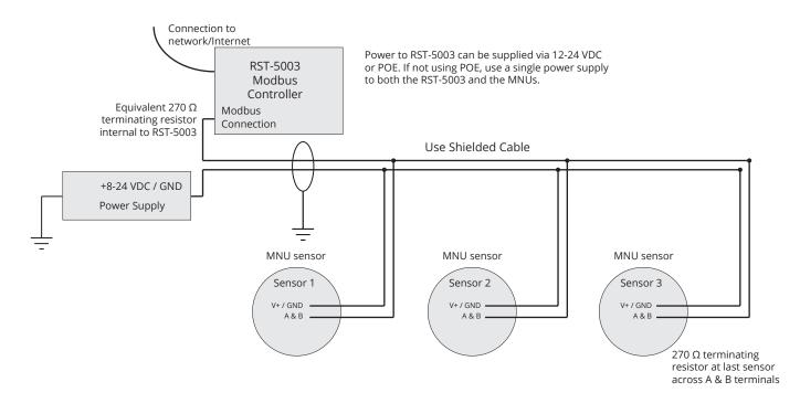
Modbus System Wiring with RST-5003 and POE or VDC Daisy Chain
